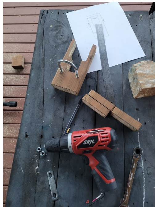
Frame with U-bolt and top pieces.
