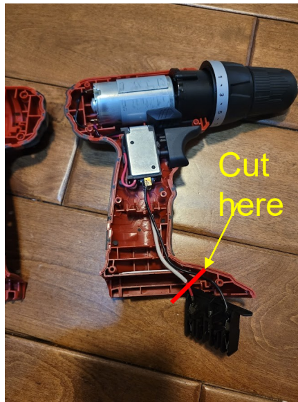
Open up and cut battery connector off.
