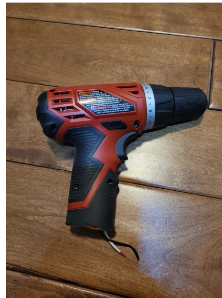
Cut off bottom battery holder and put back together.
